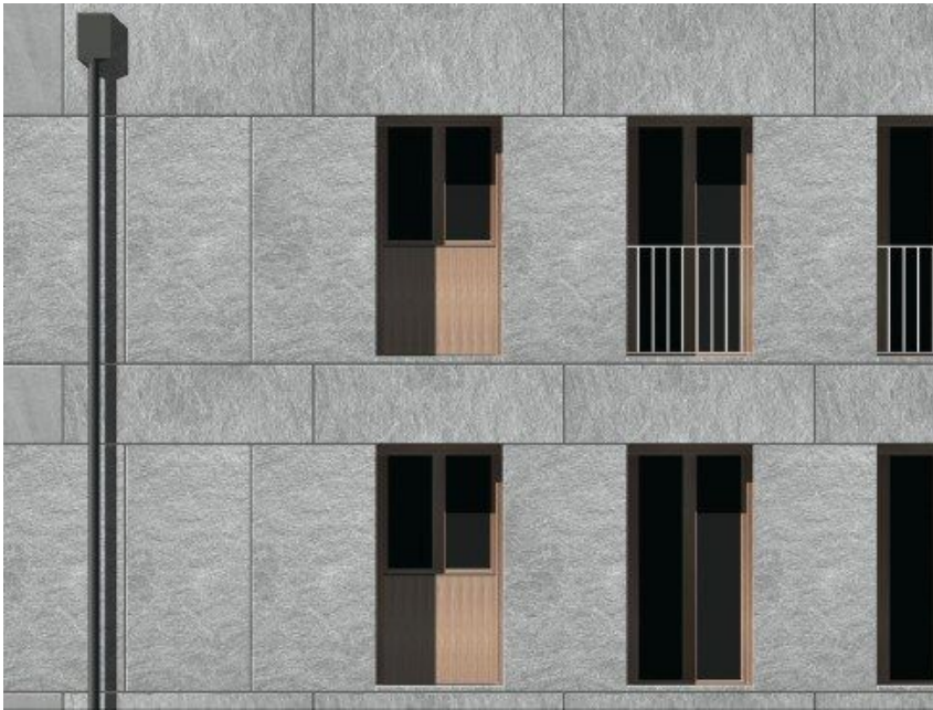
Lego-block façades with two standardized stone-formats. Computer model: Stefano Zerbi
