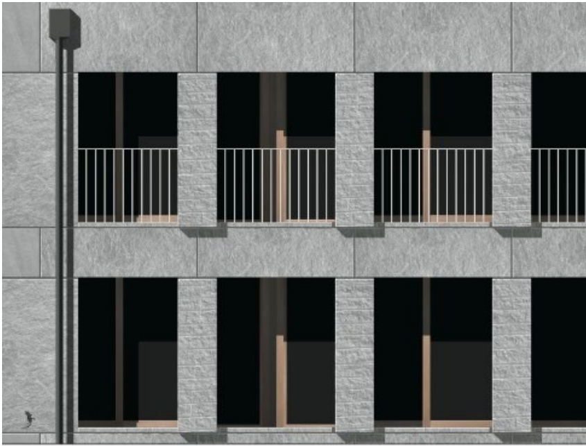
Lego-block façades with two standardized stone-formats. Computer model: Stefano Zerbi
